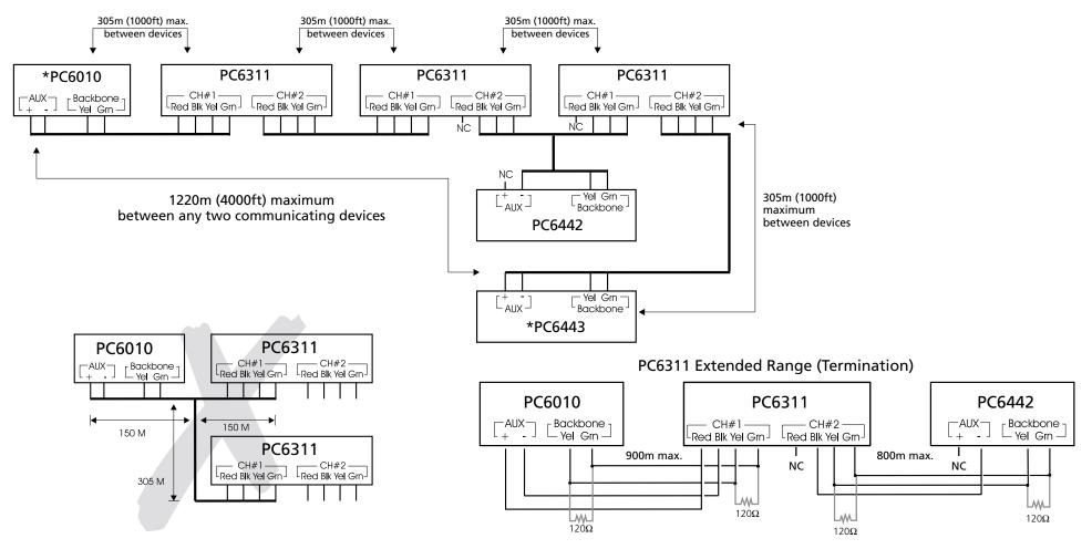
For installations where a great distance is required between two devices,  $120\Omega$  (1/4W, 5%) terminating resistors can be connected between the YEL and GRN terminals of each device as shown above. Note: For each distance indicated above, no other device can be added to the backbone.
